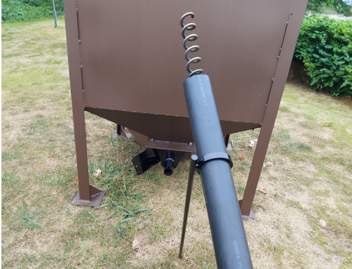
STEP 4 Slide front pipe holder post onto pipe and slide all the way to front
