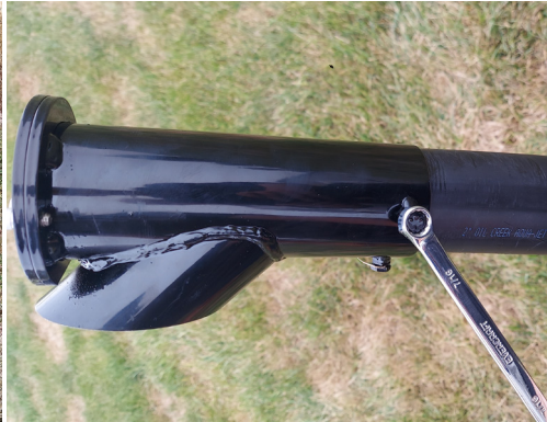
STEP 17 Loosen the two 1/4" bolts with your 7/16" wrench and turn front end so corn will drop out of bottom and then retighten bolts
