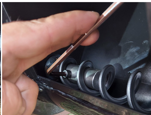
STEP 11 Insert bolt through shaft into clamp and tighten with allen wrench
