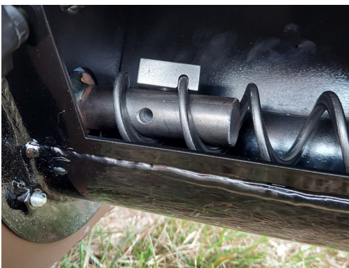
STEP 10 Slide clamp onto auger and align clamp hole with shaft hole
