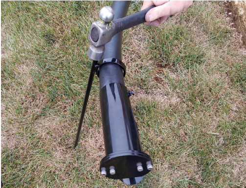
STEP 16 Install front end holder post 12" back from front and make so pipe is 12" to 16" off ground
