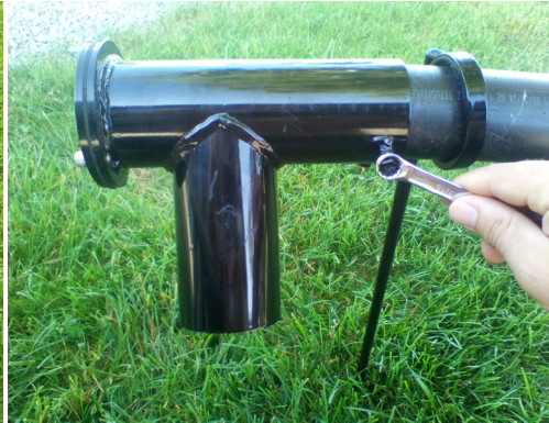
STEP 17 Loosen the two 1/4" bolts with your 7/16" wrench and turn front end so corn will drop out of both front end tubes. Must be centered!
